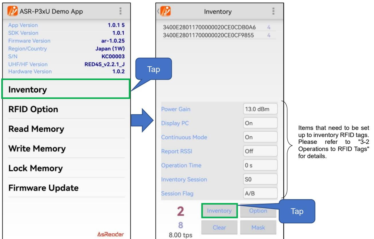
2. AsReader will continue to inventory until the set inventory stop condition is reached or the "Stop" button is tapped. (Or press and release the SCAN button again to stop the inventory.)
