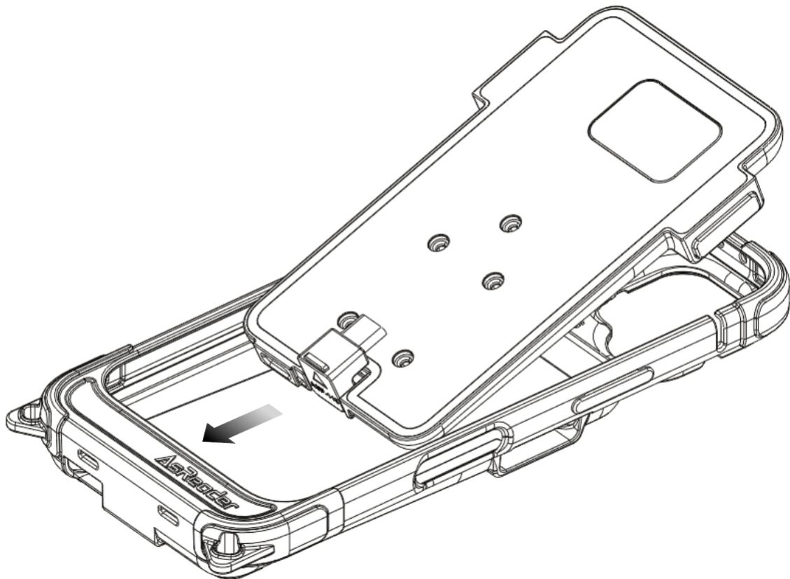
③ Bend the edge of the cover case near the camera opening.
