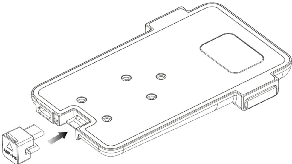
② Fit the ASR-M30S and the joint connector in the cover case.
