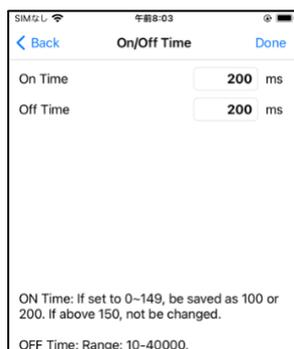
Change the On time and the Off time of RFID radio waves.
