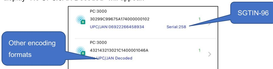
③ For UHF RF tags, tap the tag data in the list to read and write the tag.
